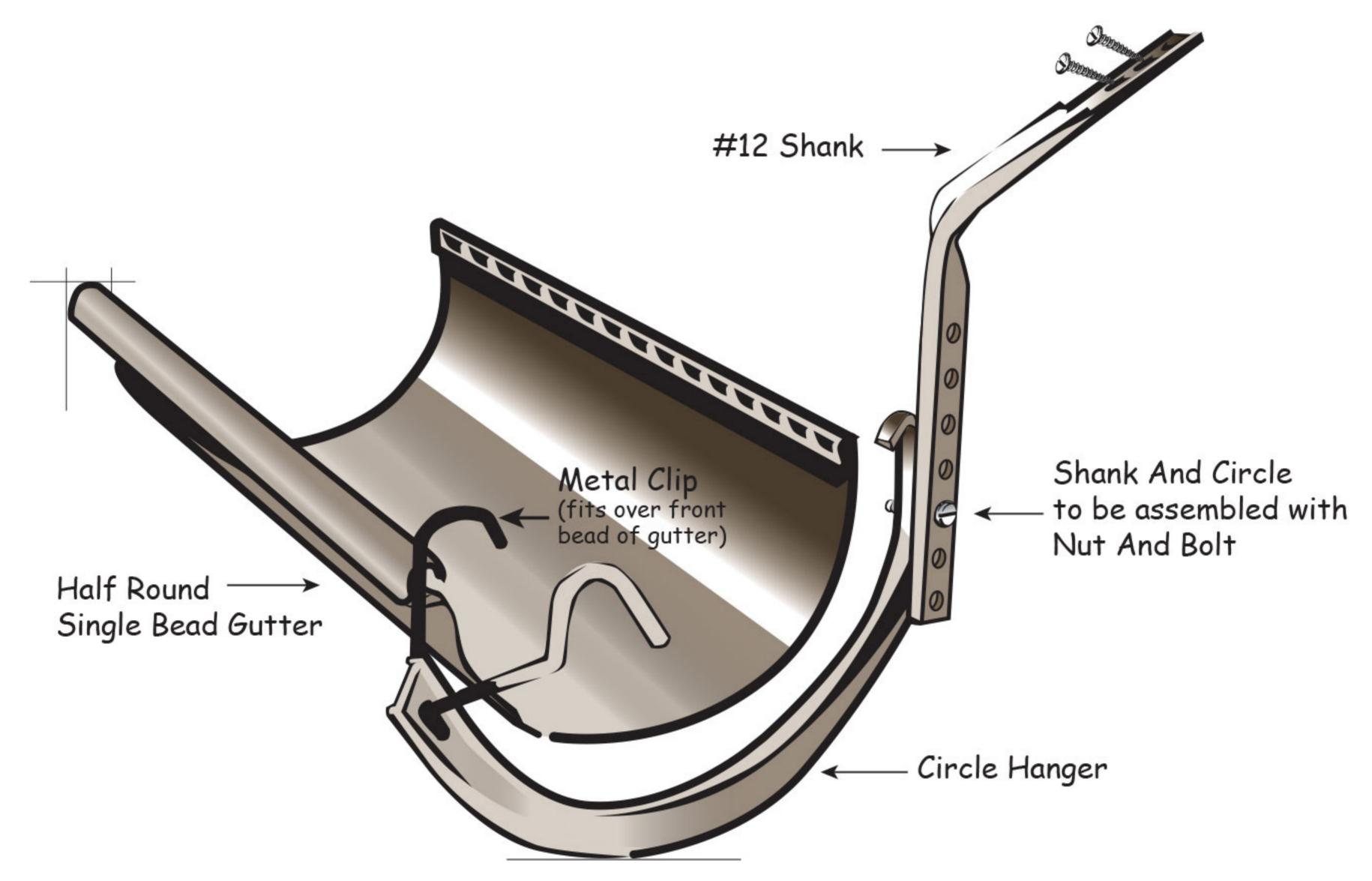
Only one hole on shank and circle will line up for nut and bolt. The flange on the circle hanger will act as a guide to stabilize the two parts together. Position nuts and bolts in lower holes of shanks to provide proper pitch in gutter.
