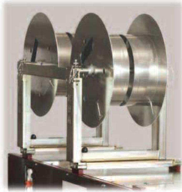
Quick release turnstile and transfer bars
