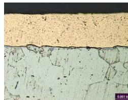
Photomicrograph of CopperPlus showing the integrity of the bond (500X)
