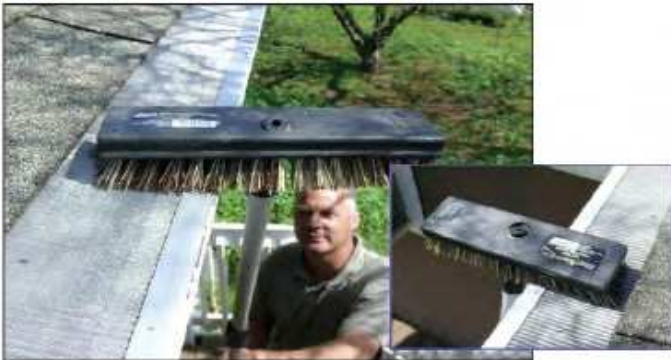
If debris ever becomes a problem where rainwater runs off the front of the gutter, you can use a brush on the end of an extension pole to brush it off.
