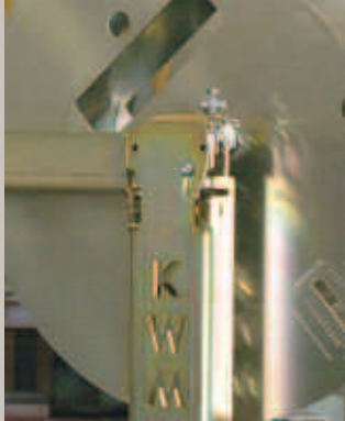
New upright, tension brake, aluminum spool and coil scale
