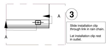
Cutaway view showing installation clip resting in outlet
