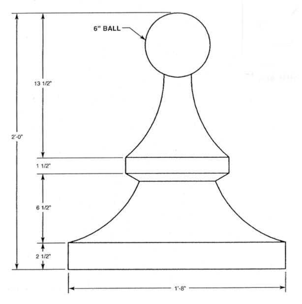
AVAILABLE COPPER MATERIALS: LEAD COATED COPPER PREWEATHERED ZINC MILL FINISHED ALUMINUM PREFINISHED ALUMINUM
