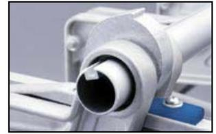
Unique Cam-Lock system clamps to the thickness of the material.
