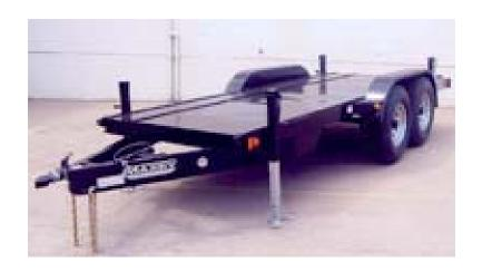
NATM Compliant, 12,000 lb. tandem axle trailer used for towing machine directly to the jobsite. Equipped with crane lifting eyes, 4 drop-foot jack stands and electric brakes w/ breakaway kit.
