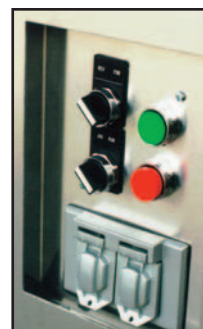
Push Button Controls
