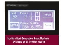
Use the touch screen to automatically control product length, add for miters, if applicable, and keep a total of daily material ran and total footage. Password protected.
