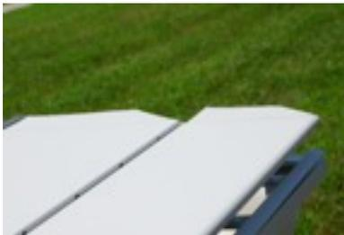
Using a quick square, make 45 degree angle markings. Leave tabs on the 45 degree angle to ensure an overlap in the seam.
